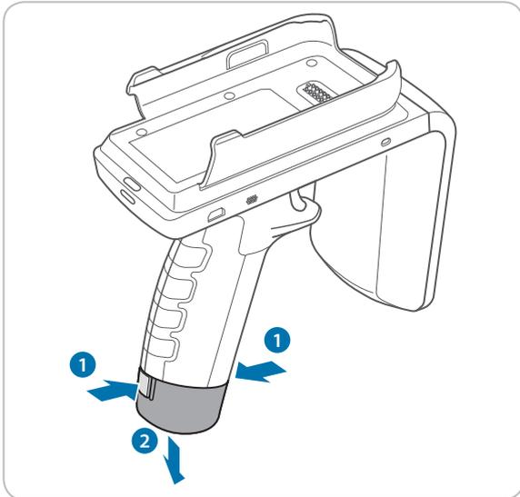
**!** Before removing the battery, turn off the power. Failure to do so may cause damage to the device.
